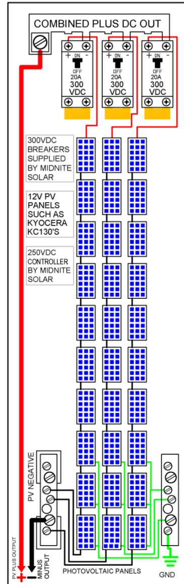
Above left: MNPV6 Disco wired with a split bus bar. A basic wiring diagram is located inside the top cover of the combiner. Additional wiring diagrams are available at [www.midnitesolar.com](http://www.midnitesolar.com) in AutoCad format. These diagrams may be downloaded and modified to represent a specific installation.
