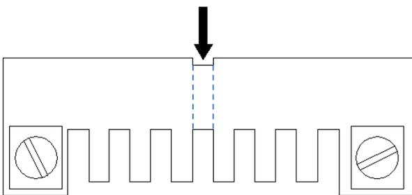
THIS PROVIDES TWO SEPARATE PLUS OUTPUTS TO FEED INTO TWO CONTROLLERS. NEGATIVE BUSBAR IS COMMON IN THIS CONDITION. CHECK TO INSURE YOUR CONTROLLER CAN USE COMMON NEGATIVES
