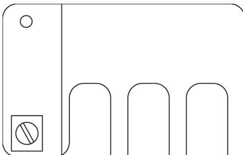
← Busbar for 300VDC Breakers. (MNPV6-250 Disco)
