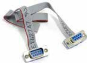
Figure 7b. Ribbon-style serial cable
