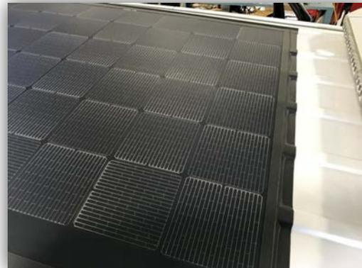
Merlin Modules to fit the contour of the vehicle roof, while providing a more uniform look.
