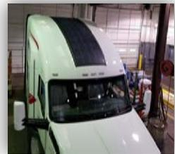
Above illustrates the full integration of Merlin Solar modules & perimeter tape with the fairings of the KW, Class 8 trucks.
