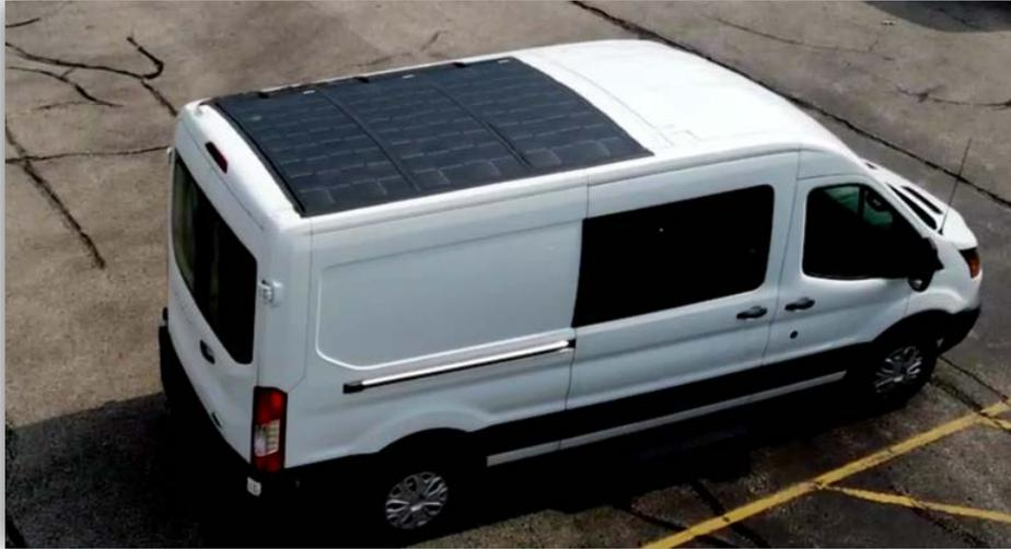
Above is example of an integrated solar array on a Ford Transit Van
