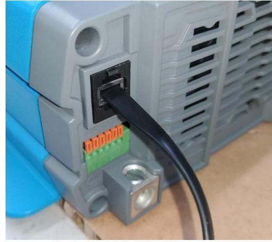
RJ-11 connect to the inverter
