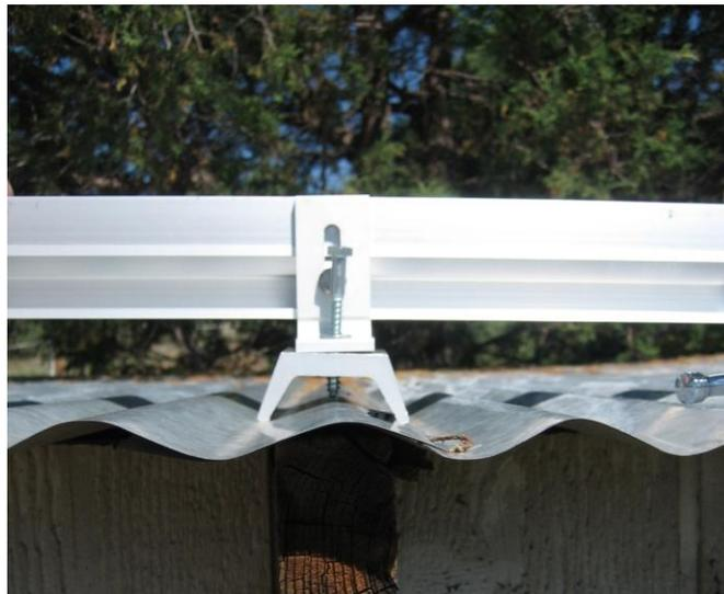
Note: the Corrugated Roof Block is designed to be installed over the high ridge of the corrugation, and be directly bolted into an underlying structural member. If a structural member, either a rafter or sufficiently strong purling, is not positioned directly under the high ridge, then additional blocking must be installed to provide a strong connection to the building's frame.
