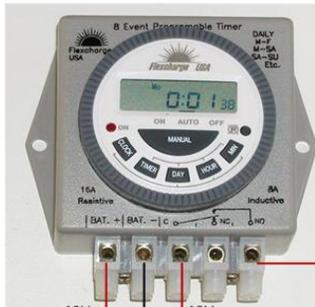
The fuse to the BAT+ terminal should be 2 amps and the fuse to the C terminal should be about 1.5 times the load amperage
